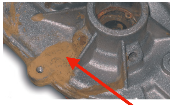
Tell Tale Sign of Water Pump Leak
